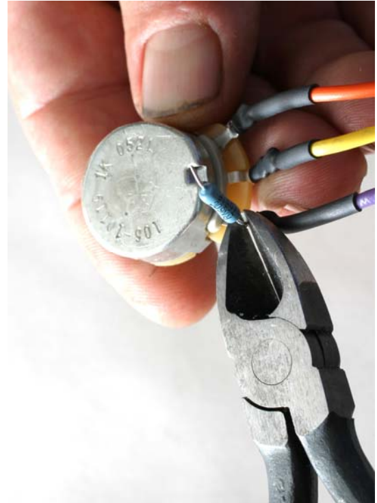
Figure 2: The resistor, visible above, is not necessary when installing the potentiometer on a newer Frymaster Thermatron-equipped fryer.
